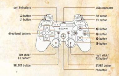
\*The L3 and R3 buttons function when the sticks are pressed.
